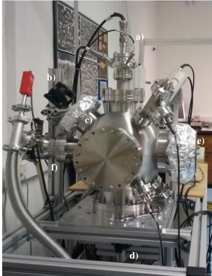
**Figure 4.7-** Picture of the setup developed for the acquisition of SEE yields (side views), showing: (a) electron gun, (b) support arm for the PMT during reflection measurements, and associated view-port (c) (covered during the measurements, except for the PMT area), (d) support arm for the PMT for transmission measurements, (e) front view port for visual control and (f) turbo pump connected to the back of the vacuum chamber.
