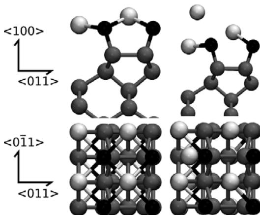
Figure 1: (Left) Top and side views of the 1 ML Li-adsorbed C(100)-(1x1):O surface. (Right) Top and side views of the 1.25 ML Li-adsorbed C(100)-(1x1):O surface, showing the distorted T3 Li position in the first monolayer.
