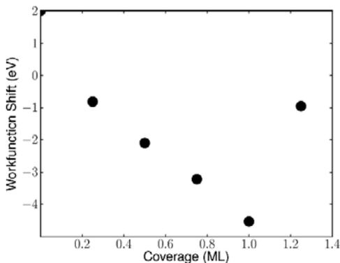
**Figure 2: Calculated workfunction shift as a function of lithium coverage for the C(100)-(1x1):O surface, relative to the clean reconstructed C(100)-(2x1) surface, workfunction 6.1 eV [11]. The bare oxygenated surface (0 ML) has a higher workfunction than the clean surface, yielding a positive shift.**
