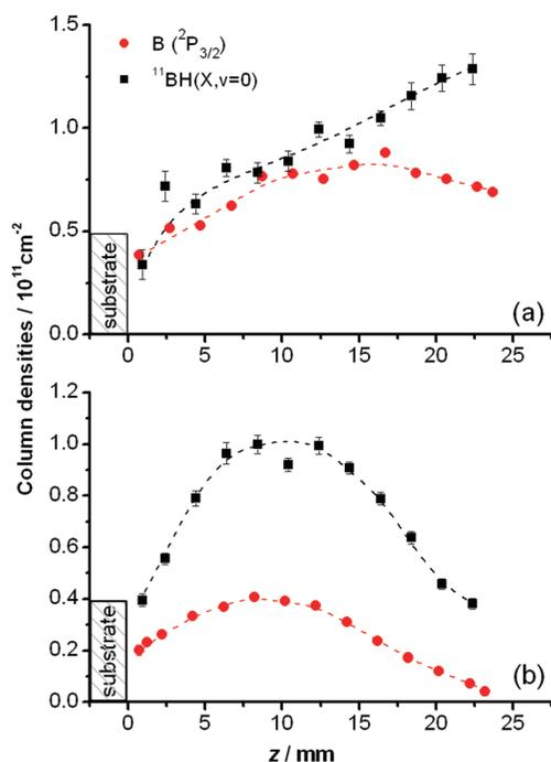
**Figure 5.**  $B(^2P_{3/2})$  and  $^{11}BH(X, v = 0)$  column densities determined by CRDS under base discharge conditions with  $F(B_2H_6) = 0.003$  and  $0.009$  sccm, respectively, plotted as functions of  $z$  at  $P =$  (a)  $1.5$  kW and (b)  $0.6$  kW.
