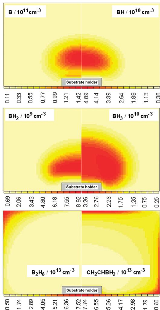
**Figure 8.** 2D( $r, z$ ) false color plots showing calculated distributions of B, BH, BH<sub>2</sub>, BH<sub>3</sub>, B<sub>2</sub>H<sub>6</sub>, and CH<sub>2</sub>CHBH<sub>2</sub> number densities under base conditions:  $P = 1.5$  kW,  $p = 150$  Torr,  $F(\text{H}_2) = 525$  sccm,  $F(\text{Ar}) = 40$  sccm,  $F(\text{CH}_4) = 25$  sccm,  $F(\text{B}_2\text{H}_6) = 0.009$  sccm, and  $F(\text{O}_2) = 0.006$  sccm.
