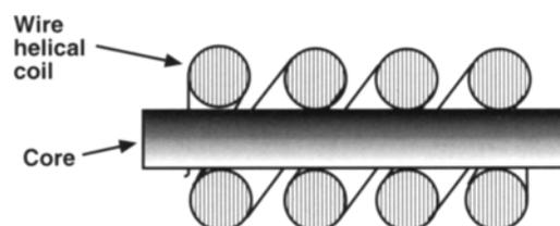
Figure 1 Schematic diagram of tungsten wire helical coil wound around a metallic or ceramic core.
