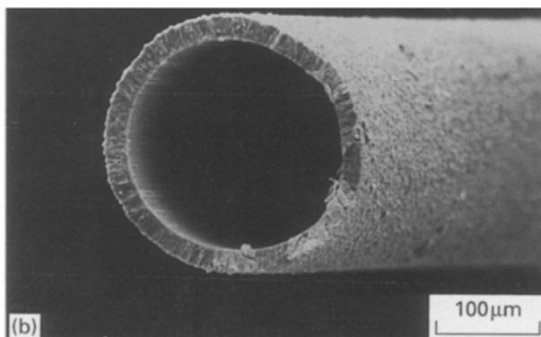
Figure 5 Scanning electron micrographs of (a) fractured end of helical coil fibre showing corrugated surfaces and (b) hollow fibre produced by etching out the core, showing smooth internal and external surfaces.
