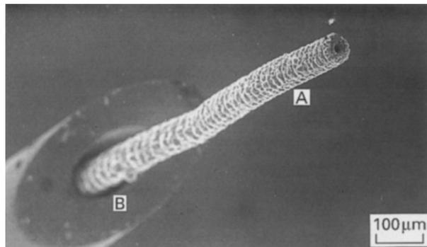
Figure 4 Scanning electron micrograph of small diameter hollow helical coil fibre at A, inserted into a hypodermic needle of internal diameter  $110 \mu\text{m}$  at B.
