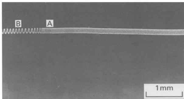
Figure 3 Scanning electron micrograph of hollow helical coil fibre at A where  $s = 2x$ , changing to diamond helical coil spring at B where  $s > 2x$ .
