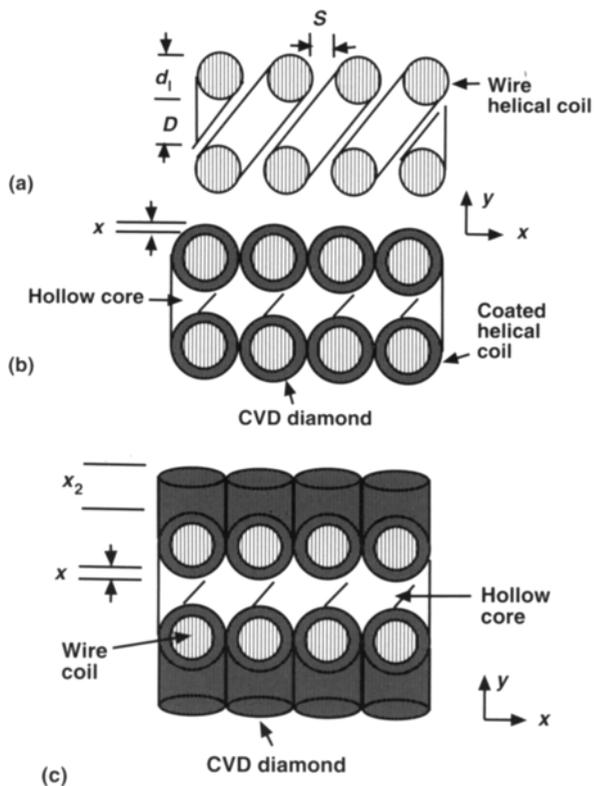
Figure 2 Schematic diagram of relaxed tungsten wire helical coil (a) after core removal, showing the dimensions of the coil, (b) after deposition of diamond to a thickness  $x = s/2$  onto the coil in time  $t = t_c$  to produce a hollow fibre and (c) diamond thickness in fibre wall,  $2x + x_2$ , after time  $t = t_c + t_f$ .
