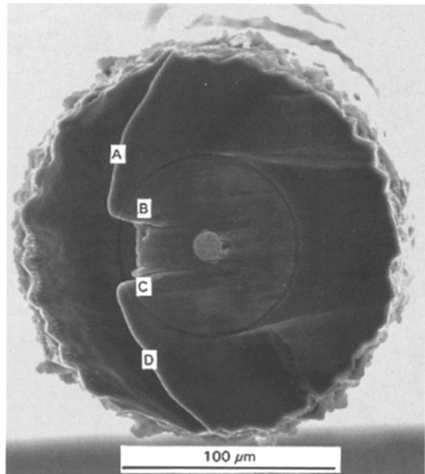
Figure 5 Plane normal to diamond-coated SiC fibre axis showing partial cut. Area BC shows where the cut has penetrated the SiC core and the cutting rate has increased relative to diamond.
