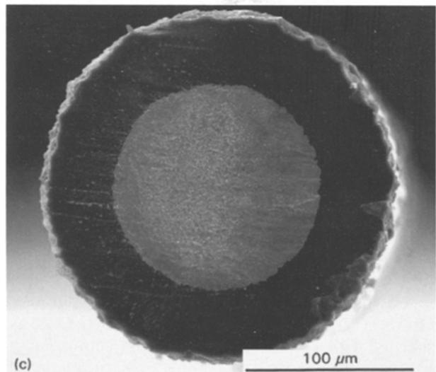
Figure 3 Scanning electron micrograph of cut diamond fibres (a) mechanically cut (b) laser cut (c) plane of laser cut normal to fibre axis.
