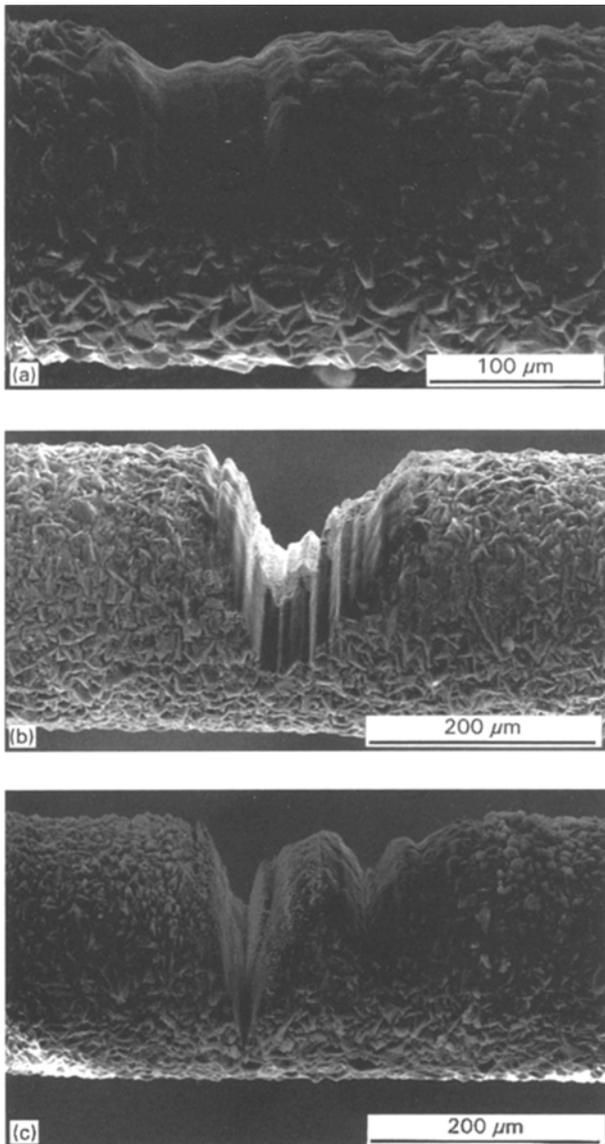
Figure 4 Partially laser-cut diamond fibres: (a) short-term cut demonstrating the polishing effect, (b) longer term with "filled-in" beam optics, (c) longer term cut with unstable resonator (doughnut) type beam.
