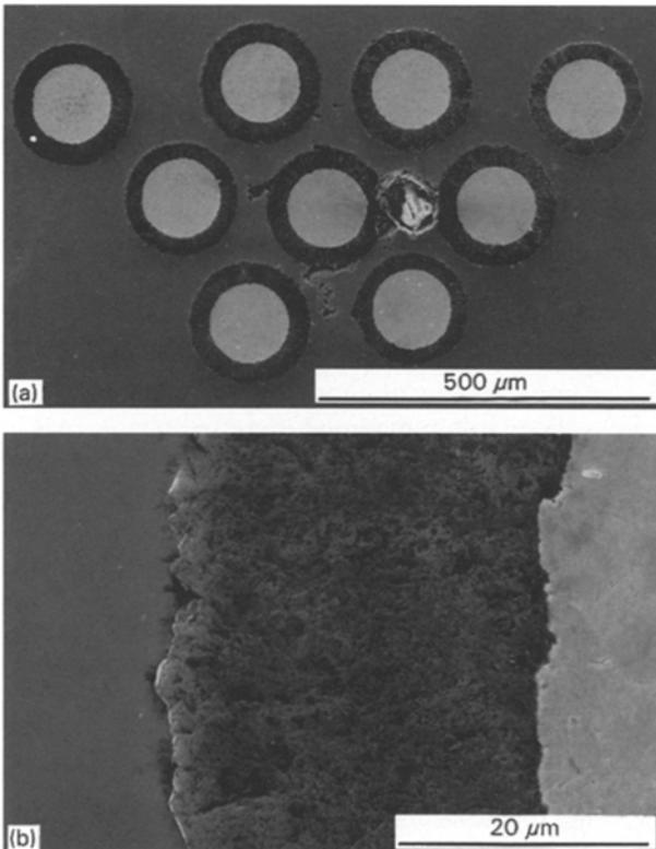
Figure 8 Scanning electron micrograph of Ti-6Al-4V/tungsten cored diamond fibre composite: (a) polished section normal to fibre axis, (b) rough abraded diamond surface in the polished section.
