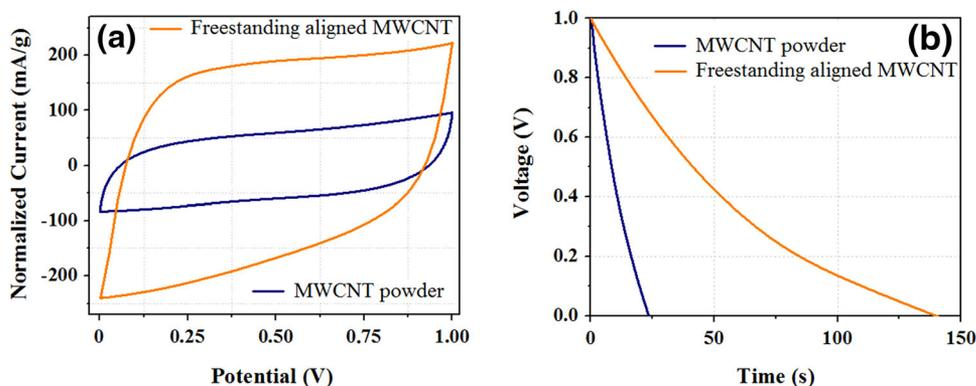
Fig. 5. (a) Cyclic voltammograms scanned at  $100 \text{ mV s}^{-1}$  and (b) constant-current at  $40 \text{ mA g}^{-1}$  from MWCNT powder and aligned freestanding materials.
