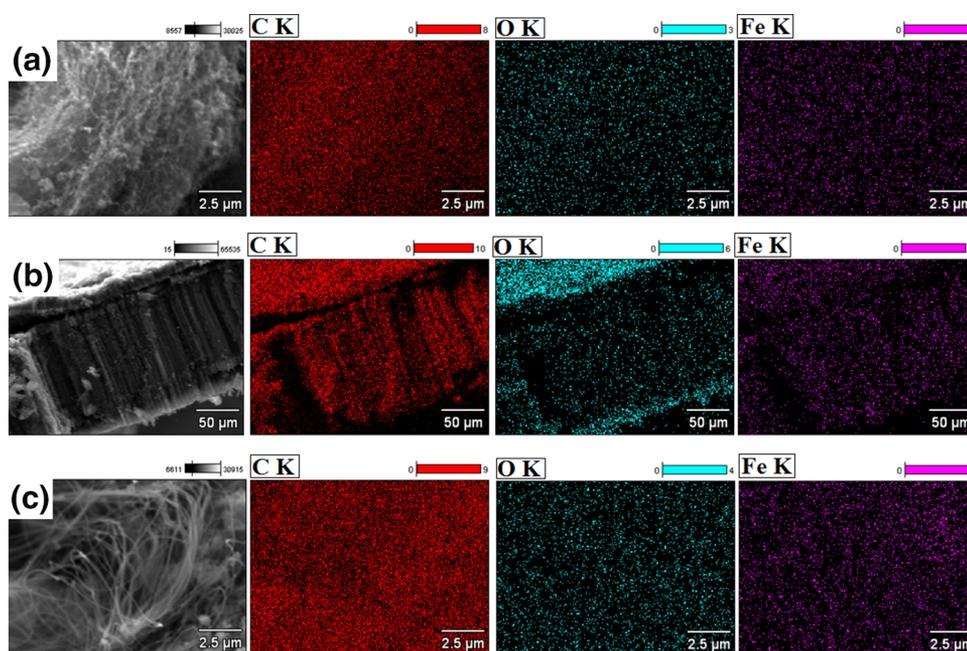
Fig. 4. EDS mapping of the surface of MWCNT (a) before and (b and c) after functionalization. The first column shows the TEM image, with columns 2–4 showing the element maps for C, O and Fe, respectively.
