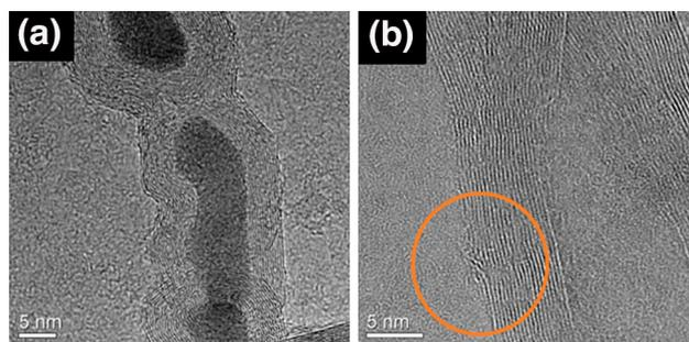
Fig. 3. TEM images of (a) as grown and (b) functionalized MWCNT samples.
