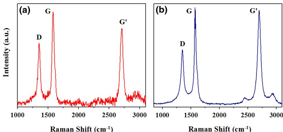
Fig. 2. Raman spectra using 514 nm laser excitation from (a) as-grown and (b) functionalized MWCNT electrodes.
