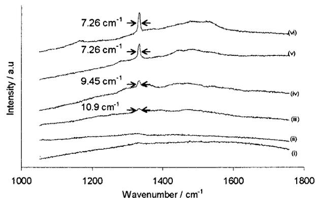
FIG. 4. Laser Raman spectra (514.5 nm excitation) of films grown in a 50% CO<sub>2</sub>/50% CH<sub>4</sub> mixture at the following substrate temperatures: (i) 435; (ii) 512; (iii) 590; (iv) 650; (v) 845; and (vi) 865 °C, other conditions as given in Fig. 2. The FWHM values for the diamond peak at 1332 cm<sup>-1</sup> are shown on each plot. The spectra have been offset vertically for clarity.
