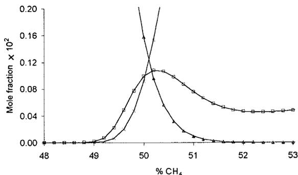
FIG. 8. Calculated species mole fractions close to the 50% CH<sub>4</sub> region, showing H<sub>2</sub>O concentrations falling and C<sub>2</sub>H<sub>2</sub> concentrations increasing. The species concentrations are equal at approximately the position where CH<sub>4</sub> concentration peaks. The data for CH<sub>4</sub> have been multiplied by a factor of 15 to fit onto the vertical scale. Key:  $\Delta$  H<sub>2</sub>O,  $\times$  C<sub>2</sub>H<sub>2</sub>,  $\square$  CH<sub>4</sub>.
