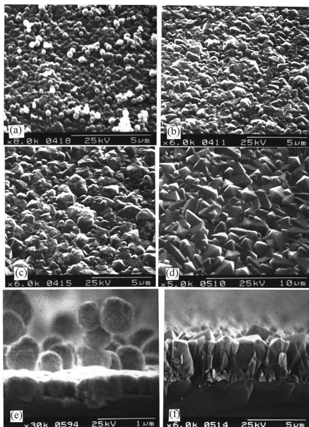
FIG. 2. Electron micrographs illustrating the increase in film crystallinity and facet size obtained with increasing substrate temperature in 50% CH<sub>4</sub>/50% CO<sub>2</sub> plasmas. Conditions: 1 kW applied microwave power, total gas flow 80 sccm, pressure 40 Torr, growth time 8 h. Substrate temperature: (a) 435; (b) 590; (c) 650; and (d) 845 °C. Cross sections of two of these films are given in (e) 435 and (f) 845 °C.
