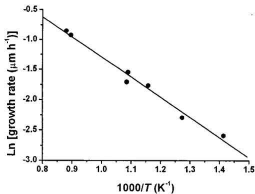
FIG. 5. Arrhenius plot of  $\ln(\text{film growth rate})$  vs inverse substrate temperature,  $1/T$ . The gradient of the fitted line gives an overall activation energy for film deposition of  $13 \text{ kJ mol}^{-1}$ .
