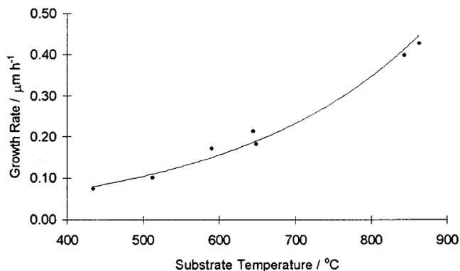
FIG. 3. Film growth rate (measured by cross-sectional SEM) vs substrate temperature for films grown in 50% CO<sub>2</sub>/50% CH<sub>4</sub> plasmas. The line is a least squares fit to an exponential function.
