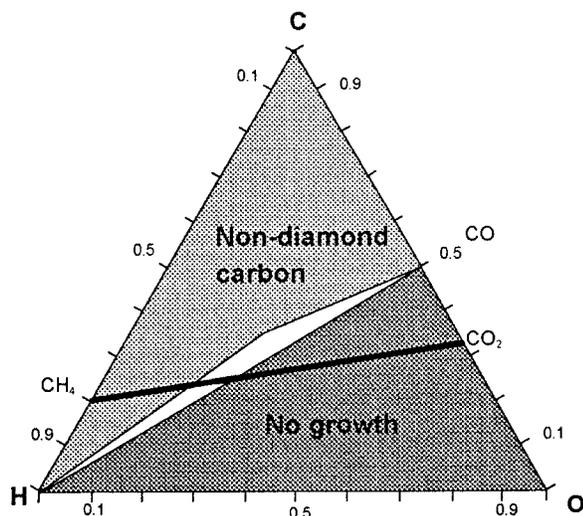
FIG. 1. Simplified atomic C-H-O diamond deposition phase diagram (see Ref. 4). The white area lying above the CO-H tie line is the experimental diamond growth domain. The thick CH<sub>4</sub>-CO<sub>2</sub> tie line corresponds to the full range of CO<sub>2</sub>/CH<sub>4</sub> gas mixtures used in this work.
