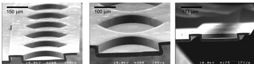
FIG. 3. SEM images of the free-standing nanocrystalline diamond lenses after silicon etch and removal.
