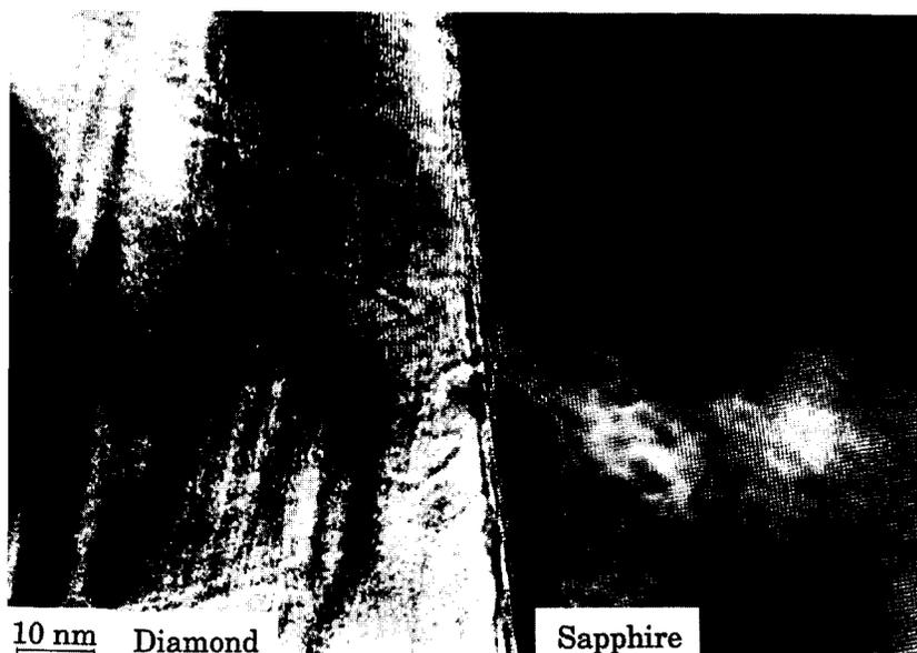
Fig. 5. High resolution TEM cross-section through the diamond/sapphire interface showing the intimate contact between the two crystal lattices without any obvious amorphous interlayer.
