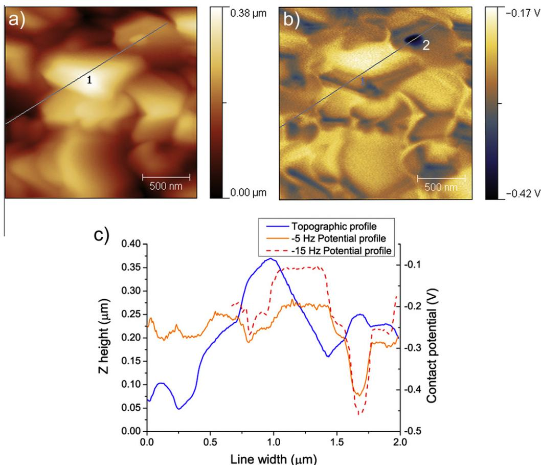
**Figure 3.** Images of specimen B1 obtained using KPM, (a) surface topography map, (b) contact potential difference map with '2' representing a possible graphitic feature on the diamond surface, (c) line profiles corresponding to line 1 in (a) and (b), demonstrating variations in contact potential across the surface of the specimen.
