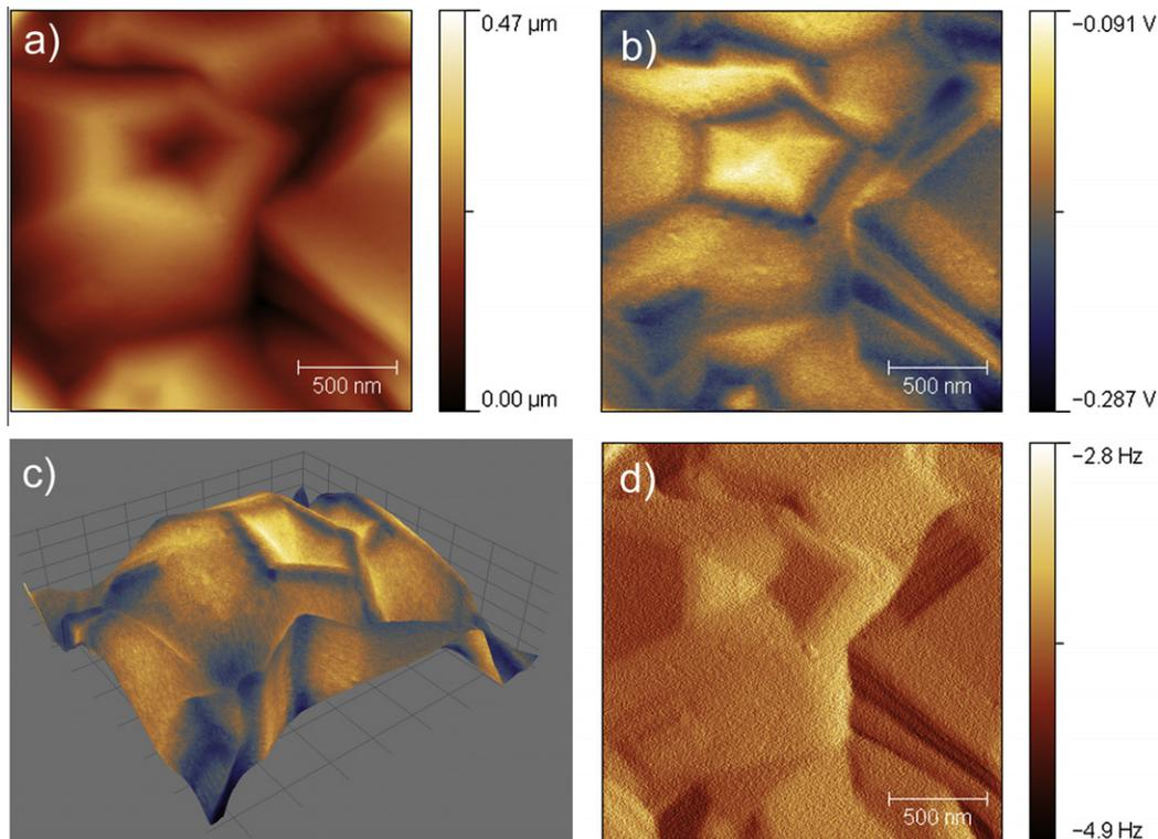
**Figure 2.** Images of specimen B2 obtained using KPM. (a) surface topography map, (b) contact potential difference map, (c) three-dimensional topographic map overlaid with contact potential map, and (d) df (frequency shift) image.
