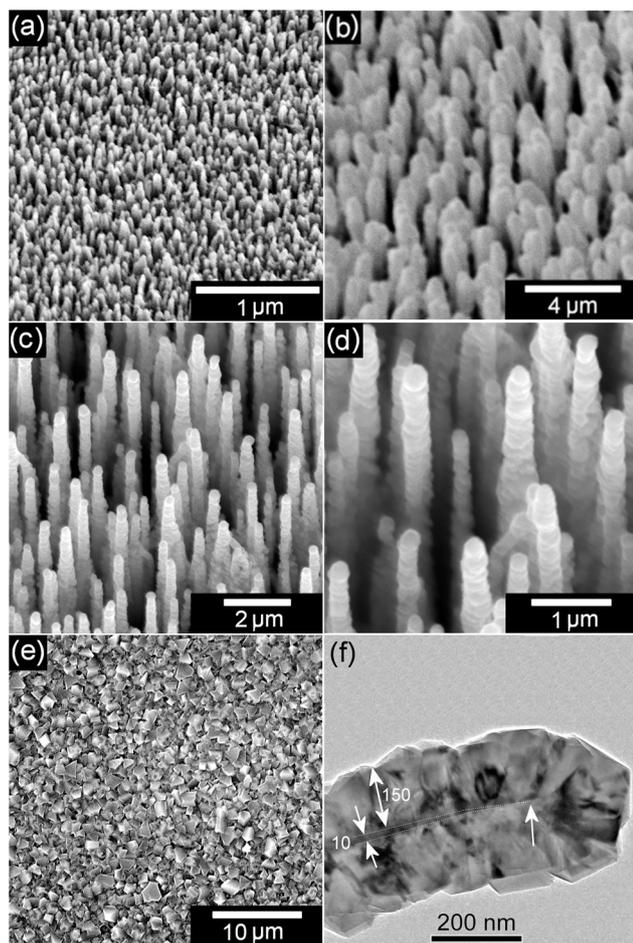
**Fig. 2** SEM images of the various bD samples (a) short needles, (b) medium needles, (c, d) long needles, (e) the 'flat' diamond control sample and (f) high-resolution TEM image of the end of a bD needle showing core-shell structure. Measurements are in nm. The diamond film thickness is  $\sim 150$  nm, while the Si needle core is  $\sim 10$  nm at the left of the picture, tapering to a point at about midway across shown by the right arrow.
