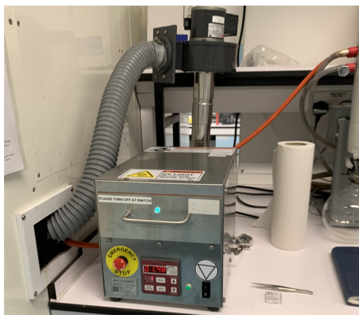
Figure 17: An image showing the UV ozone cracker used to perform oxygen termination.
