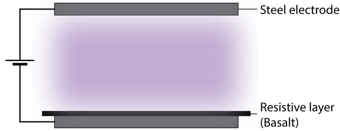
Figure 1.10: Schematic of a Resistive Boundary Discharge device, which can be operated in a glow discharge mode using AC or DC. 49,87
