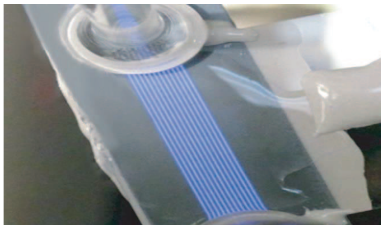
Figure 1.14. Photograph of a 12-channel microplasma ozone generator operating in 1 atmosphere of \text{O}_2 . 88
