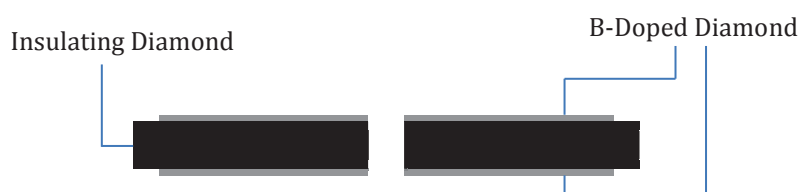
Figure 1.17. A diagram of the MHCD type device fabricated solely from diamond by Mitea et al. 125
