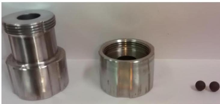
Figure 14. Grinding jar and steel beads
