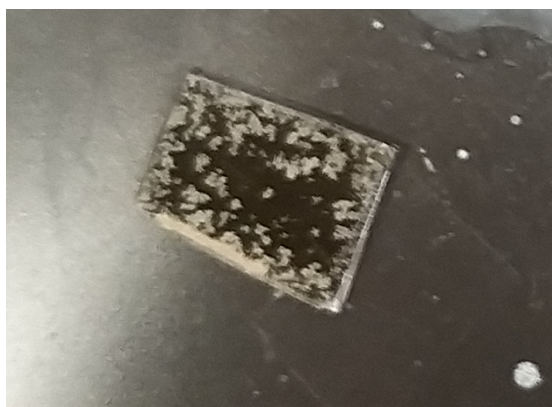
Fig.33 - One of the bDi samples showing clear markings after deposition and heating.
