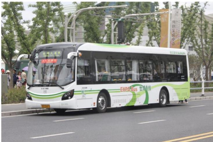
Figure 9: A fully supercapacitor-powered 'Capabus', premiered at the Shanghai Expo 2010.
