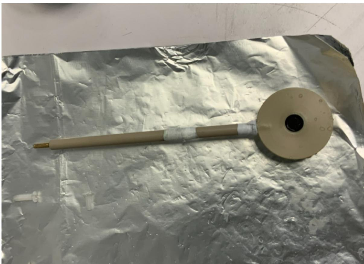
**Figure 4.1.** The electrode holder for f-BDD and EBL-BDD samples. The sample being held here is an f-BDD sample.
