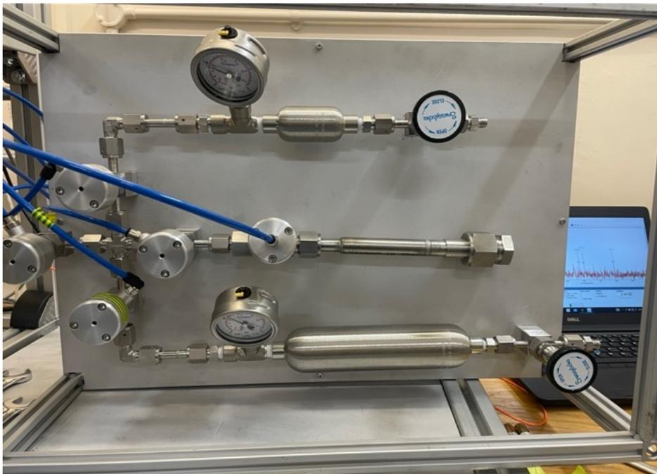
*Figure 18. The fully assembled gas board configuration with the methane accumulator (Top), Vial breaking assembly (Middle) and hydrogen accumulator (Bottom) installed with pneumatics connected.*
