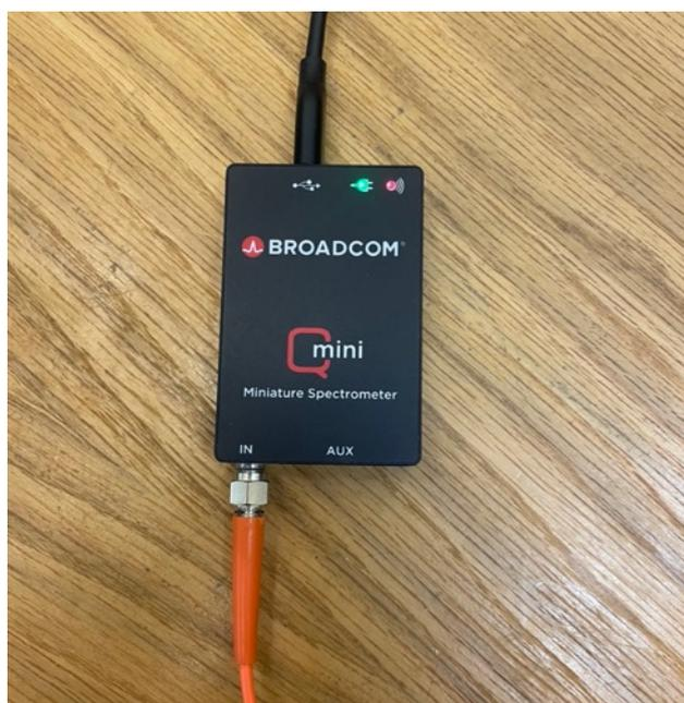
**Figure 14.** The Broadcom Qmini spectrometer used to monitor how the optical emission spectrum varies during the deposition process.
