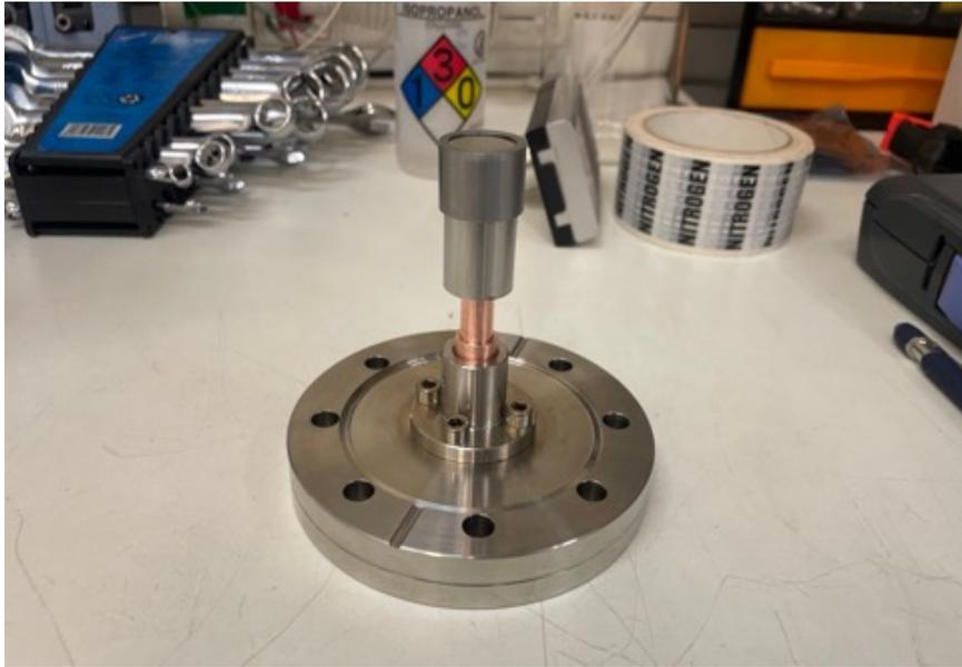
*Figure 17. The molybdenum anode with the newly fitted bezel holding the substrate in place on top of the copper electrode mount.*
