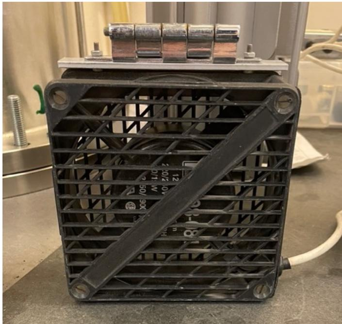
*Figure 26. The fan used in the unsuccessful attempt to cool the mini-PDR reaction chamber during test VII.*
