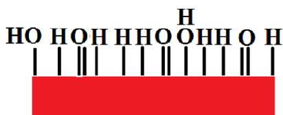
**Figure 2.2.3:** Cartoon diagram of how O-terminated sample would look like under incomplete oxygenation treatment, with the presence of H-termination.
