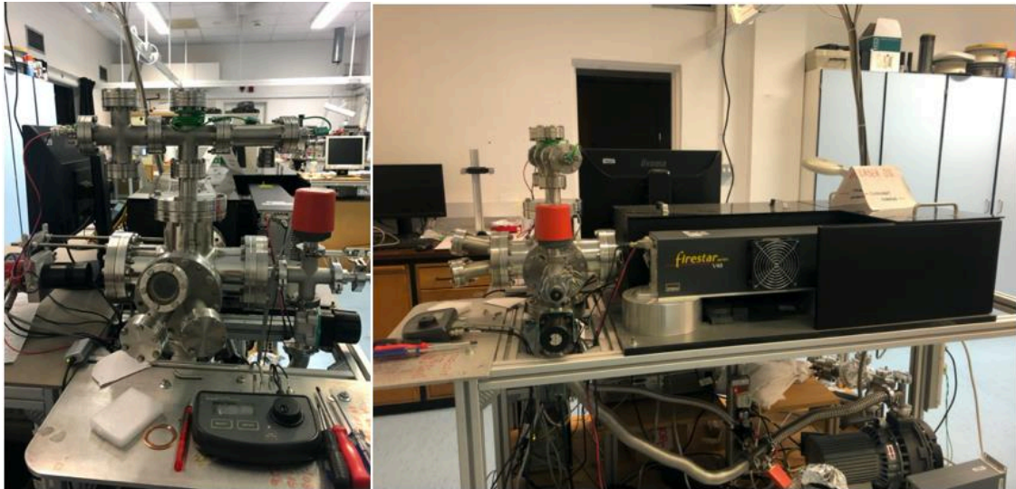
Figure 16 - Thermionic testing equipment in the University of Bristol Diamond lab.
