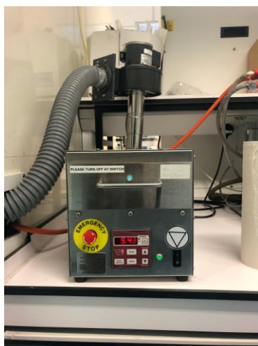
Figure 14 - Ozonolysis machine at University of Bristol.
