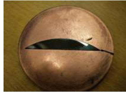
**Figure 30.** NSSi3 after deposition. The right point was placed at the edge of the molybdenum deposition plate with the straight edge running along the plate's diameter.
