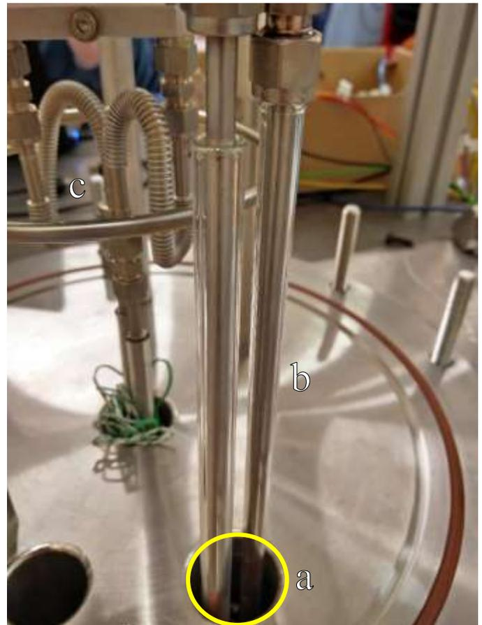
**Figure 14.** The feed through in working order after final modifications were completed. The small feed through opening (a), highlighted in yellow, was leading to the issues with arcing, while the glass rods (b) and the flexible coolant pipes (c) were installed to counter this issue.
