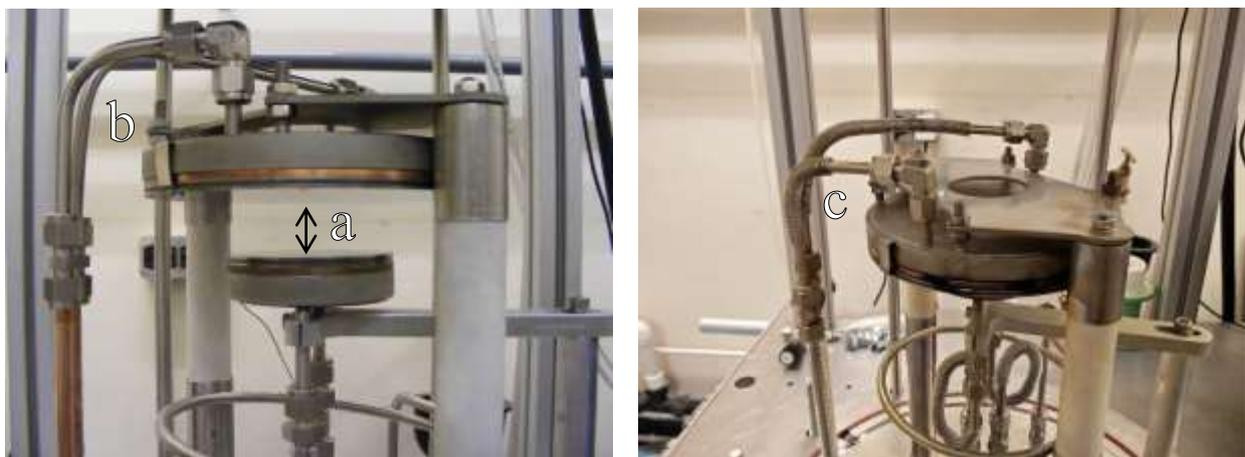
**Figure 15.** The initial deposition plates set up with the large electrode gap and inflexible water cooling pipers (left), and the final set up with the shorter interelectrode gap (not shown) and the new flexible piping for plate movement (right).
