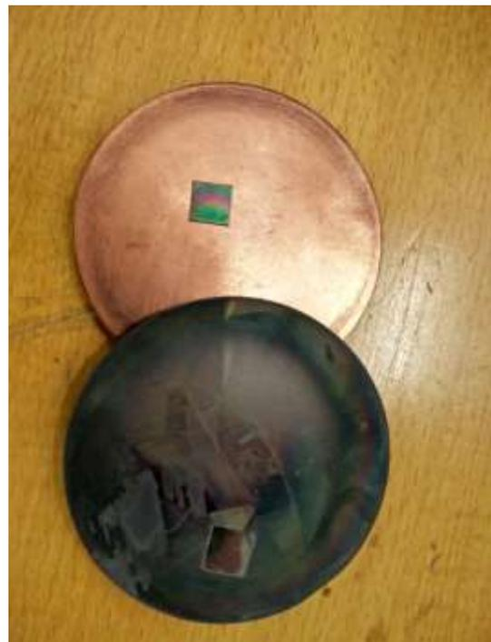
**Figure 35.** Produced films from Ex4 showing SSi4 and the molybdenum deposition plate.
