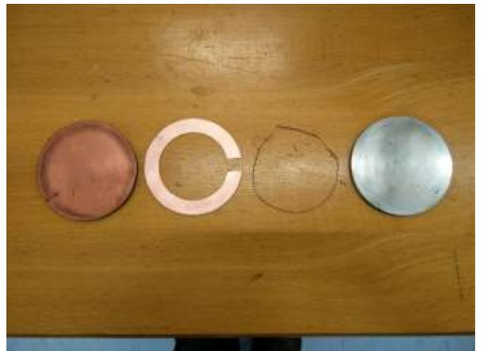
**Figure 16.** The different cooling systems utilized on the PDC PA-CVD reactor. From left to right; the full 3 mm thick copper spacer with thermocouple slot cut out, the 1 mm thick copper 'C', the 0.5 mm thick tantalum wire, and the molybdenum deposition plate.
