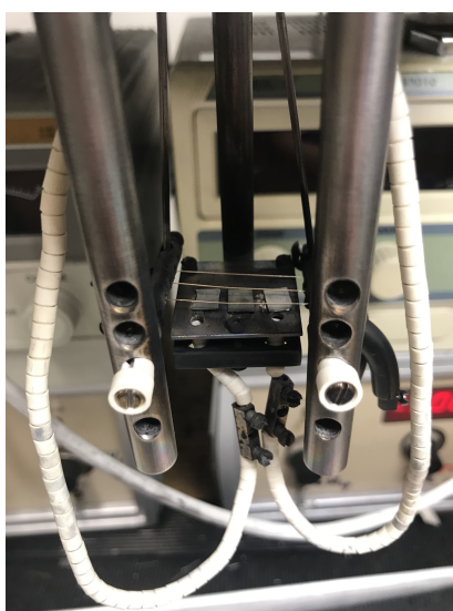
FIGURE 2.2: Black diamond samples under tantalum wire filaments, having grown for 30 minutes.
