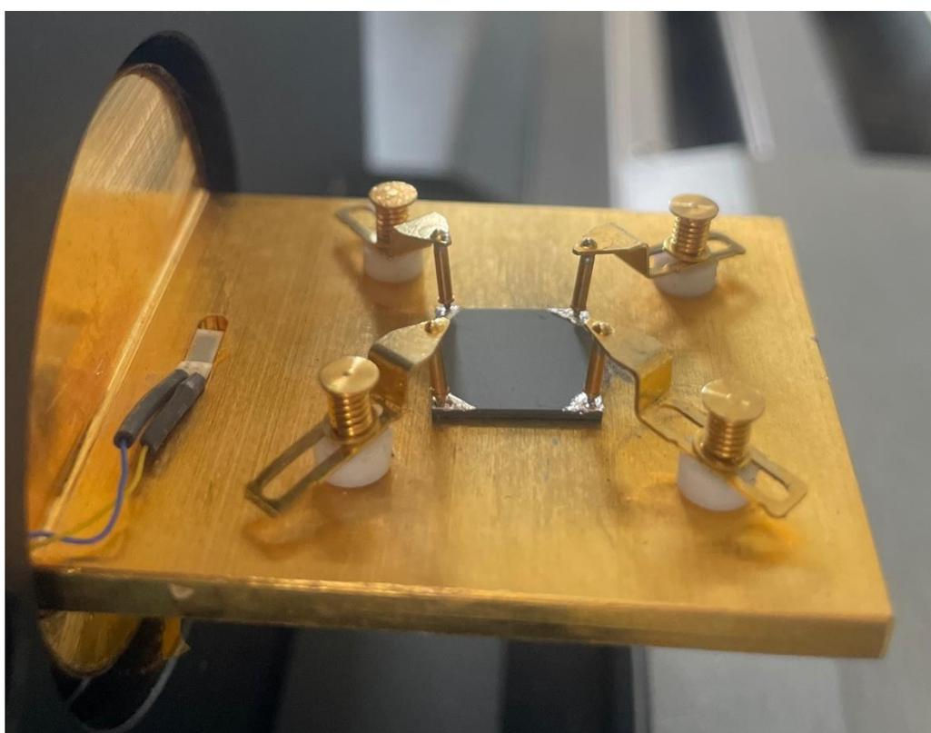
Figure 24- A photograph of a sample with indium contacts loaded into the Hall effect measurement system
