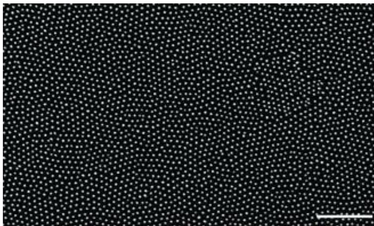
Figure 5. A top down SEM image of the Cicada wing, showing the distribution of the nano-pillars.<sup>34</sup>
