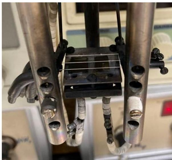
*Figure 13. Black silicon samples below tantalum wire filaments.*
