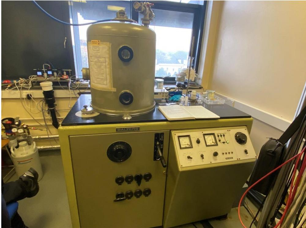
Figure 10: A photo of the Balzers CVD Coating System.
