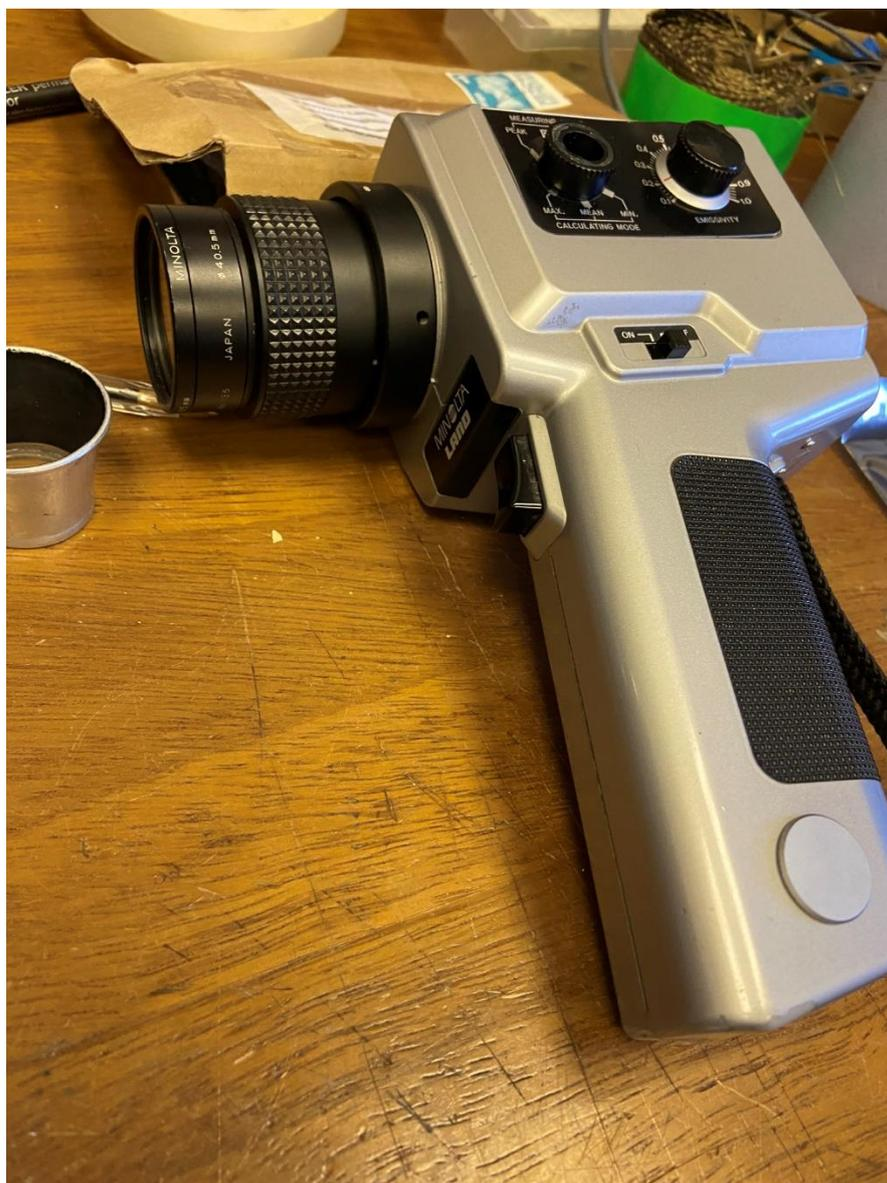
Figure 14: A photo of the Minolta infra-red thermometer, which was used to measure the temperature of the cathode, plasma and substrate.
