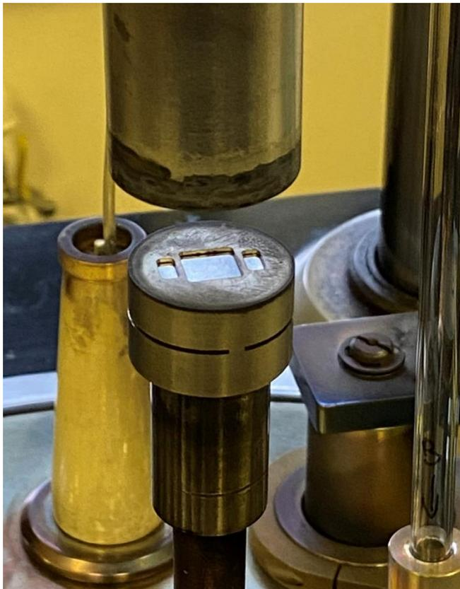
Figure 13: A close-up photo of the set-up for the molybdenum reaction. A molybdenum substrate was placed on top of the anode. A mask was placed on top of the substrate, allowing the reaction to occur only at the square hole and the two small rectangular holes on both sides.
