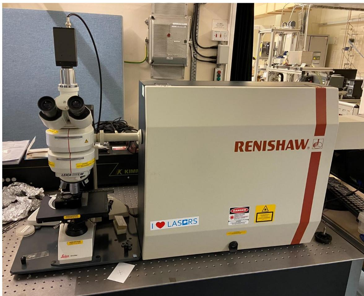
*Figure 17: A photo of the Renishaw Raman spectrometer, with LEICA confocal microscope installed.*
