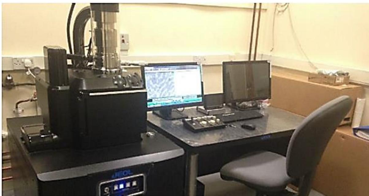
**Figure 2.6: An image of the JEOL IT300 Scanning Electron Microscope used in this study.<sup>13</sup>**
