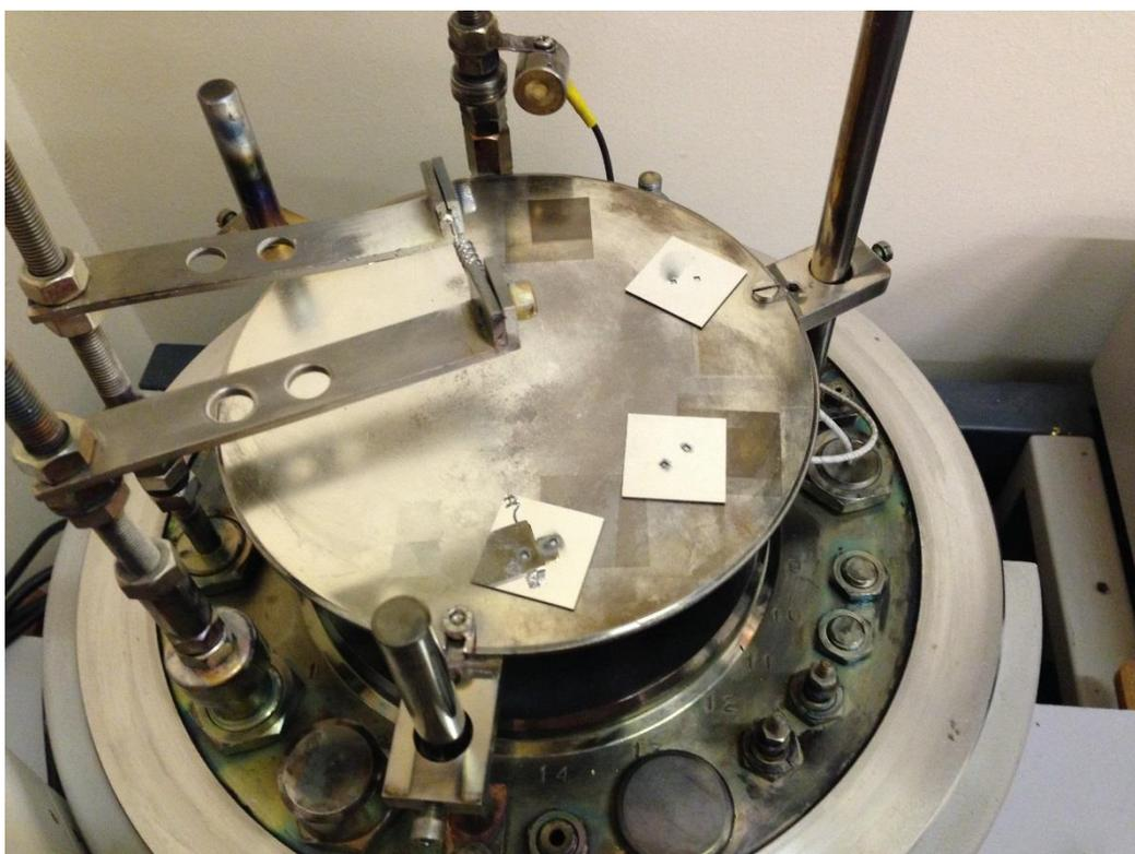
**Figure 2.6: Schematic and photograph of the inside the bell jar evaporator showing the masks with  $1 \times 1 \text{ mm}^2$  holes with the diamond sample underneath. The tungsten filament and silver wire can also be viewed.**
