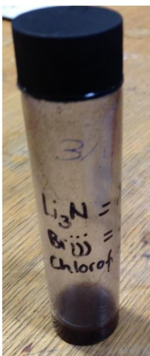
**Figure 2.3:** Li<sub>3</sub>N solution, prepared by forming a suspension of Li<sub>3</sub>N powder and chloroform (1% w/v polyoxy in chloroform).
