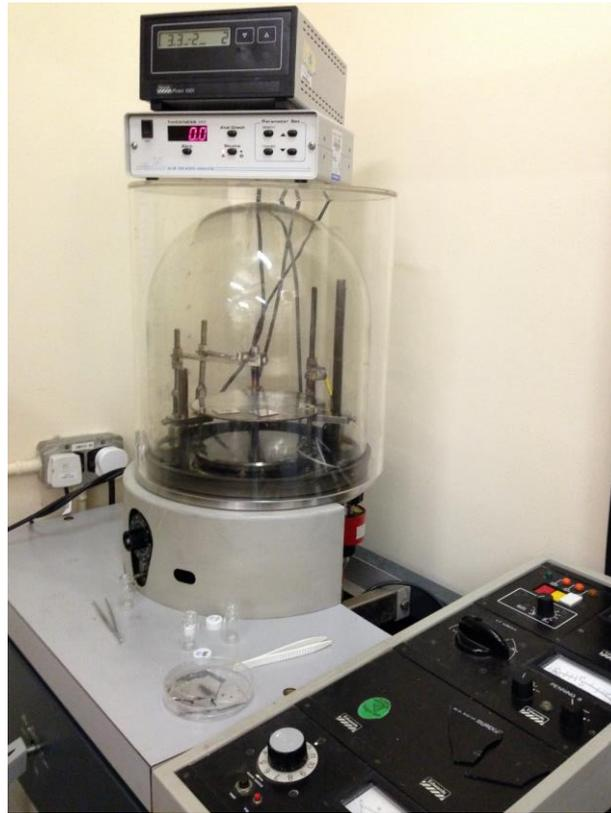
**Figure 2.5: The ball jar evaporator, located in the Diamond laboratory, University of Bristol with the thickness monitor and the Edwards Pirani 1001 pressure monitor on top of the bell jar.**
