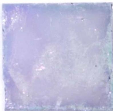
**Figure 45:** Photograph of the diamond membrane after a 7 min NCD deposition, before being removed from the AlN substrate.
