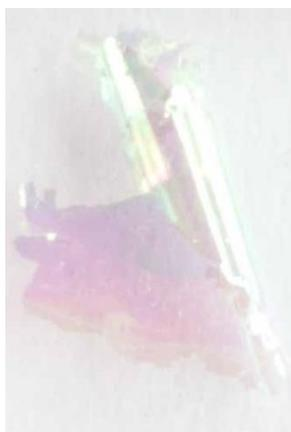
**Figure 44:** Photograph of the free-standing, nanocrystalline diamond film after a 7 min deposition.
