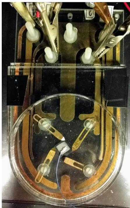
FIGURE 2.7: Aerial photograph of the van der Pauw setup used. The device in the photograph is an unwanted test sample and does not have the four metal probes in contact with the ohmic contacts as usually employed for analysis.
