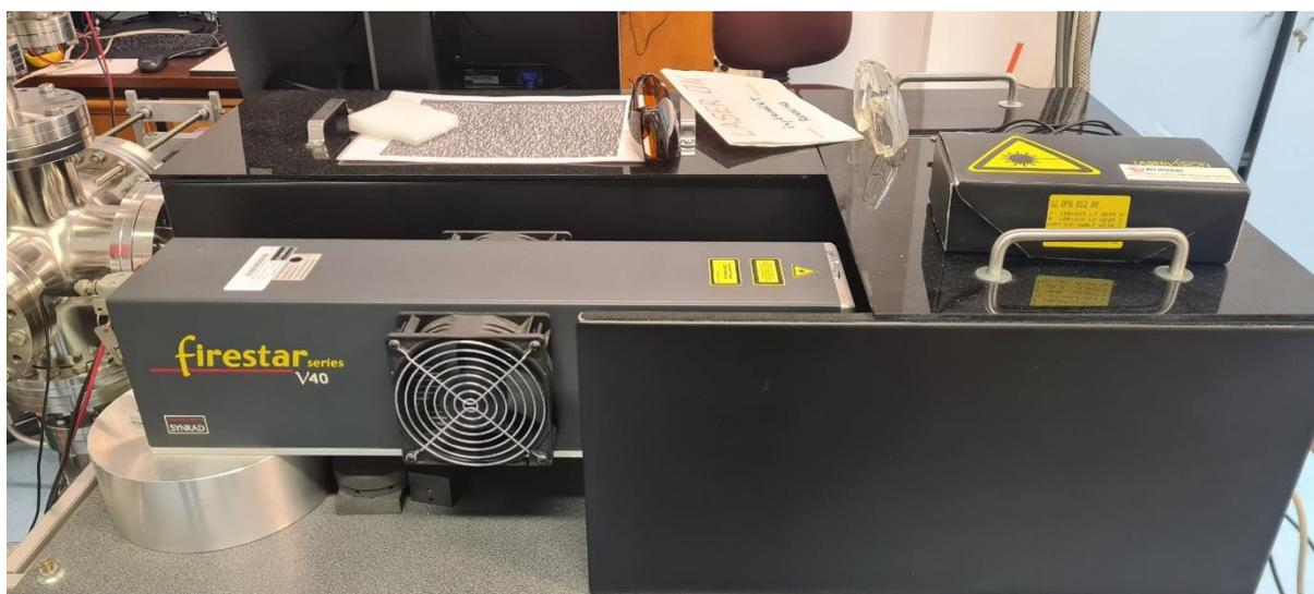
**Figure 9.8:** Photograph of the Synrad FSV40KFD, Firestar laser.
