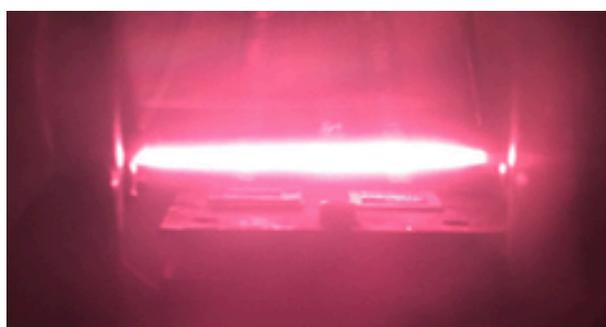
Figure 3.7: Photo of HF-CVD BDD deposition. Two substrates are visible under the glowing-hot tantalum filaments.
