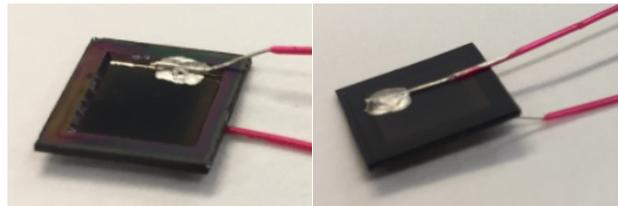
Figure 3.2: Photograph showing sample; (left) Si window-frame side-up; (right) Growth-side (GS) of i-diamond layer up.
