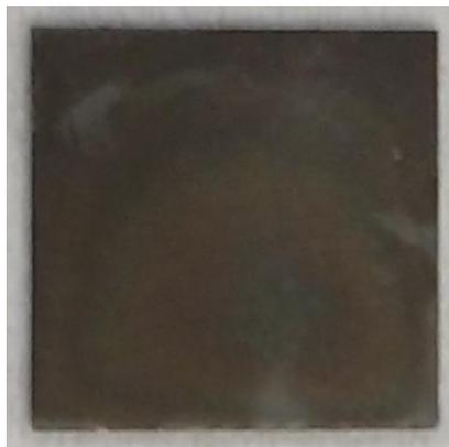
***Figure 32: Photograph of DFMo 2 after oxygen termination, aluminium deposition and a 10 min wet etch with 1.2 M HCl. The patches that are lighter are indicative of a thinner aluminium coating.***
