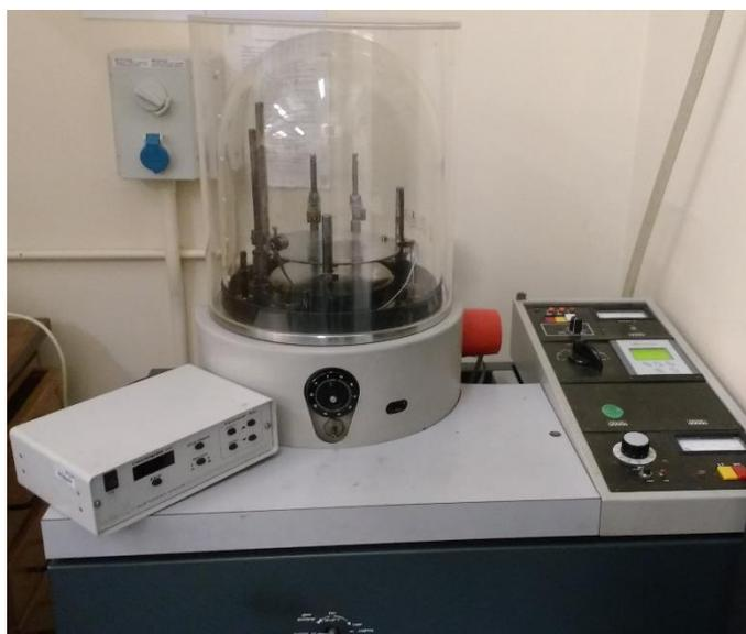
**Figure 13: Edwards bell jar evaporator used for aluminium evaporation.**
