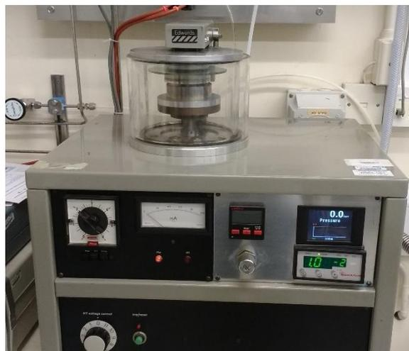
**Figure 12: Converted Edwards sputter coater used for oxygen termination.**
