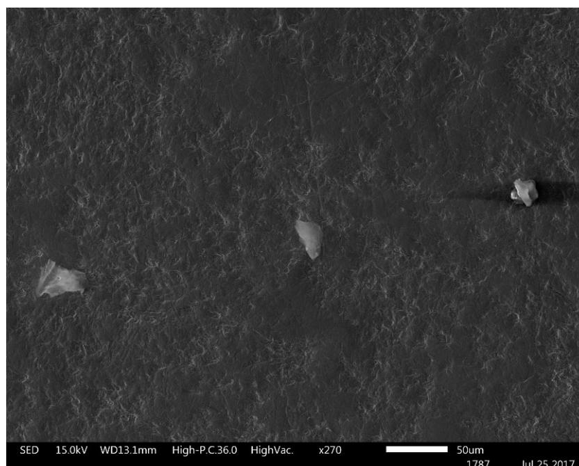
Figure 3.9: SEM image of the surface of sample 2. The material on the surface is dirt, rather than diamond nucleation, shown to give perspective of the surface.
