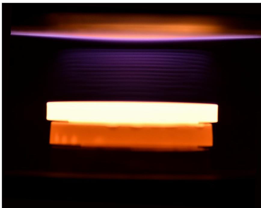
Figure 3.1: H<sub>2</sub> “cleaning plasma” – 200 Torr, 3 kW, with 3 substrates each separated by a wire spacer ring. The lowest substrate, the anode and plasma are difficult to see due to the brightness of the top substrate.
