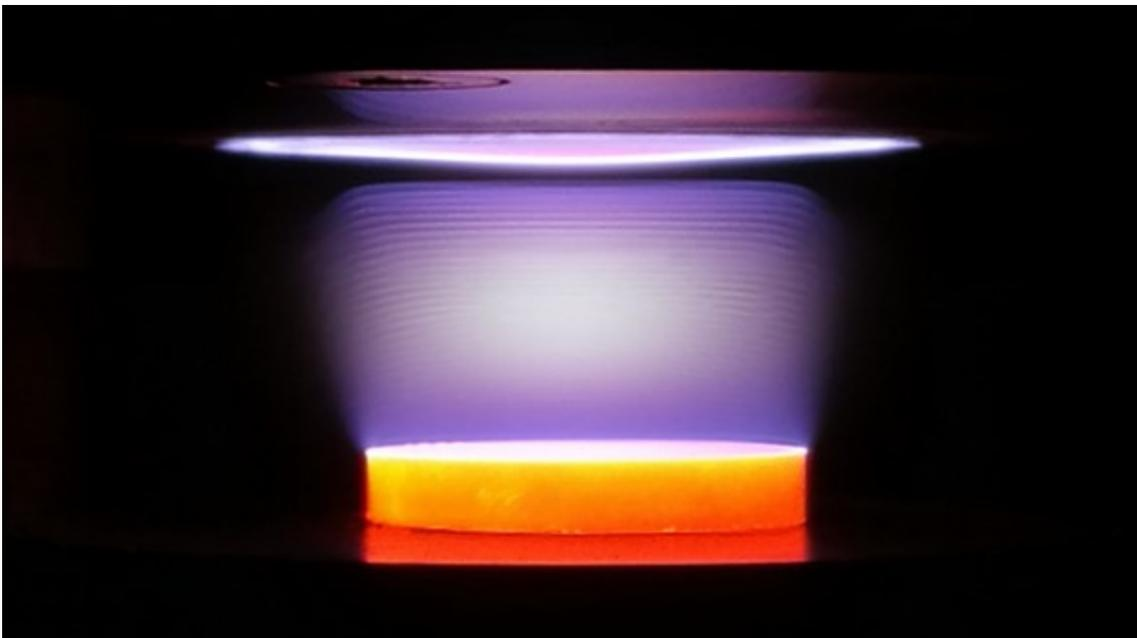
Figure 3.5: Photograph of a CH<sub>4</sub>/H<sub>2</sub> plasma at 200 Torr, 3.3 kW, 12 minutes after the addition of CH<sub>4</sub>. The ring spacer was 0.5 mm diameter, and as such, the space between the anode and the substrate is harder to see.
