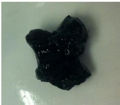
**Figure 32:** Nanodiamond hydrogel before washing with water.
