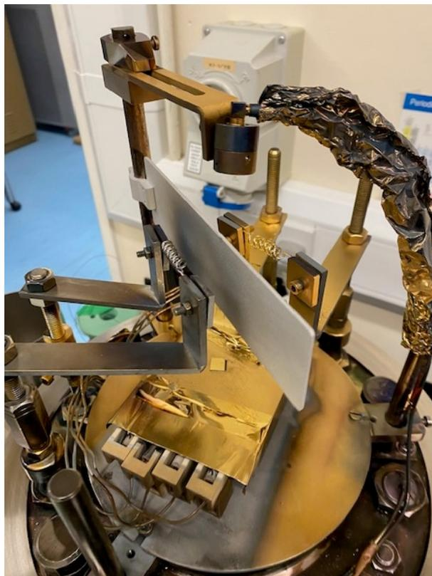
Figure 1.10: Photograph of the evaporator system. Loaded in the coiled filaments is gold on the right and aluminium on the left.
