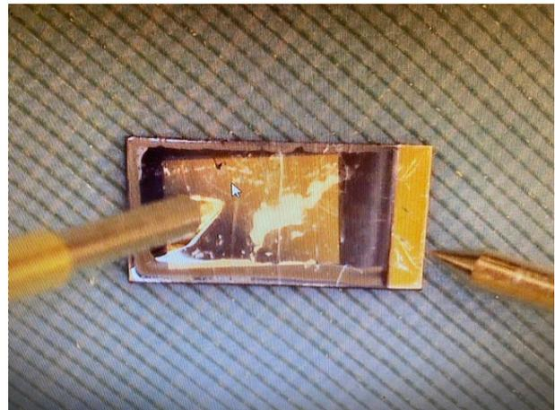
Figure 2.2: Photograph of the 2-point probe system in use. Probes are placed as far away from contacts as possible to ensure equal measurements between runs.
