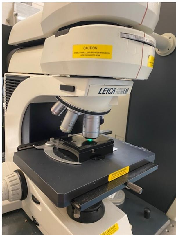
Figure 2.1: Photograph of the Raman spectrometer in use. Samples are loaded onto the stage, focused with visible light then illuminated with laser light to take the spectrum.
