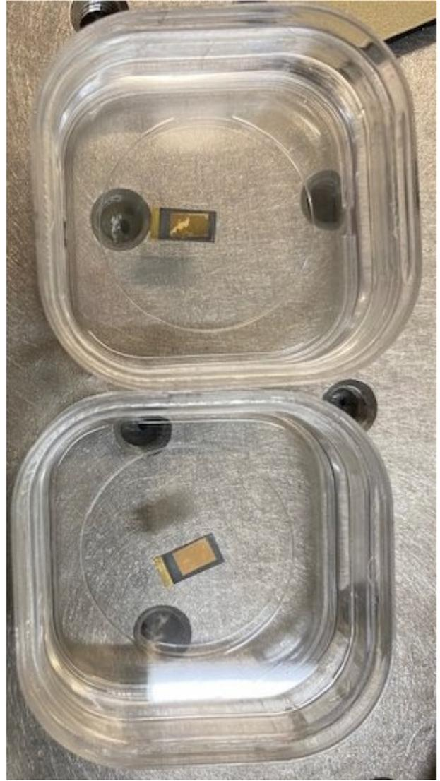
Figure 3.15: Photo of the diodes diode immediately after metallisation. Above is the hot filament grown diode and below the microwave grown diode.
