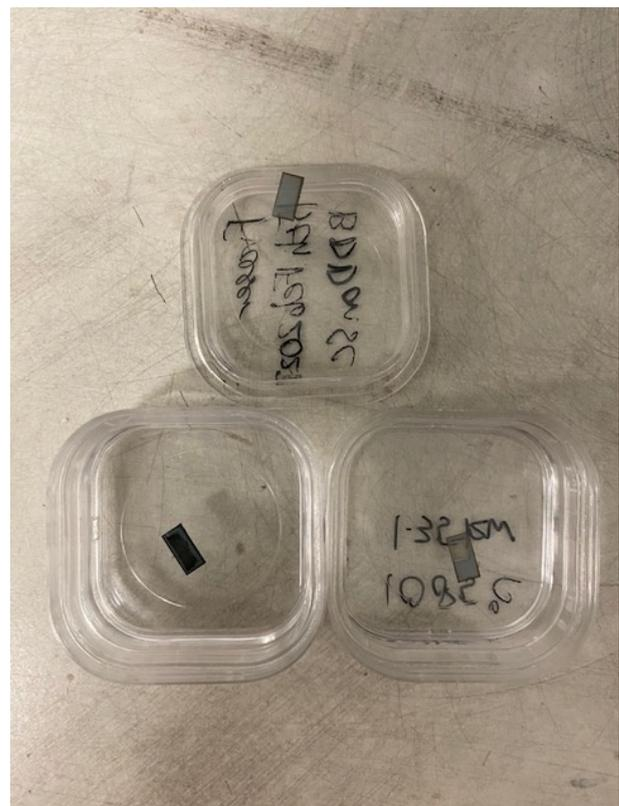
Figure 3.11: Photo of the 3 samples grown: bottom left is the hot filament sample, top is layer (6) and bottom right is the masked layer (6) sample. Notice how much darker the hot filament sample is, implying a greater concentration of boron.
