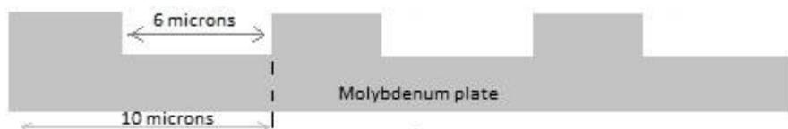
Figure 29 - Optimal Mo plate for absorbing CO<sub>2</sub> laser beam.
