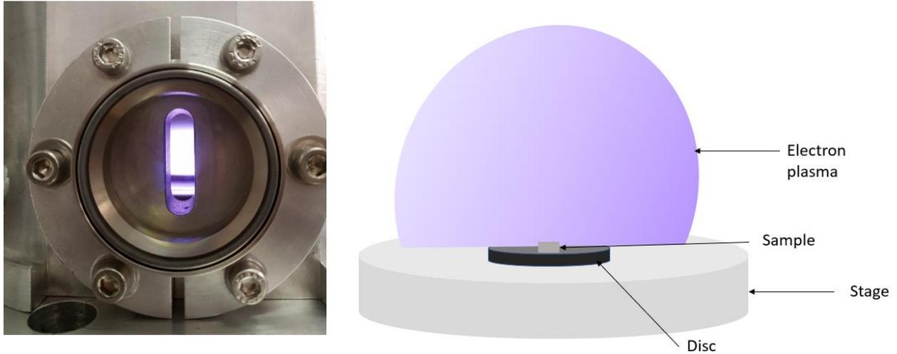
**Figure 17.** The left picture shows a view of the plasma during a H termination. The right diagram shows a simplified set up of the sample inside the vacuum chamber surrounded by the electron plasma.
