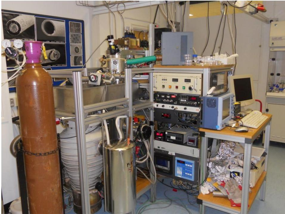
**Figure 4.2:** A photograph of the MWCVD reactor in the Bristol Diamond Group.
