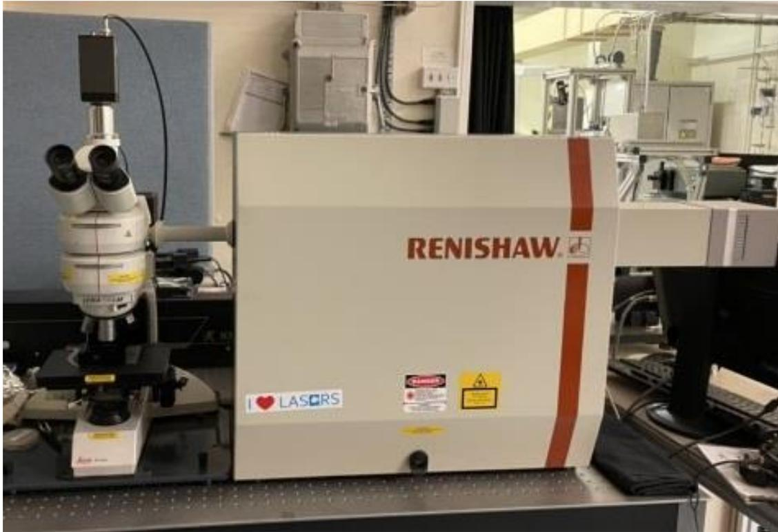
Figure 21 Raman spectroscopy kit.
