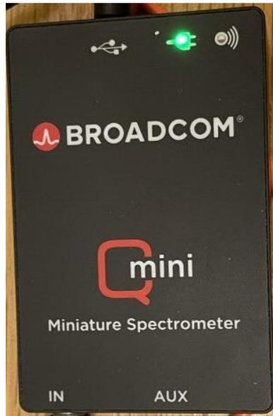
**Figure 20** Optical emission spectrometer used in this research.
