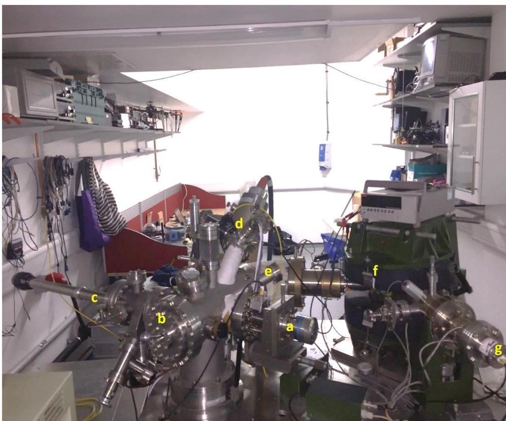
**Figure 3.13.** Photograph of the SIMS instrument. a) sample stage manipulator; b) analysis chamber; c) entry chamber; d) Ga<sup>+</sup> ion gun; e) electrostatic analyser; f) magnetic sector; g) detector
