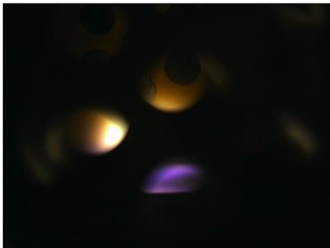
**Figure F.9:** Side image of plasma sustained with a gas composition of 4.4% CH<sub>4</sub>, 7 % Ar; balance of H<sub>2</sub> at a pressure of 150 Torr sustained at 1.25 kW.
