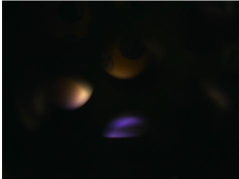
**Figure F.8:** Side image of plasma sustained with a gas composition of 4.4% CH<sub>4</sub>, 7 % Ar; balance of H<sub>2</sub> at a pressure of 150 Torr sustained at 1.0 kW.
