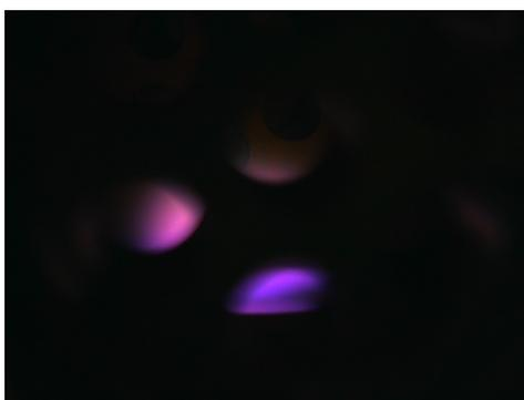
**Figure F.4:** Side image of plasma sustained with a gas composition of 7 % Ar; balance of H<sub>2</sub> at a pressure of 150 Torr sustained at 1.5 kW.
