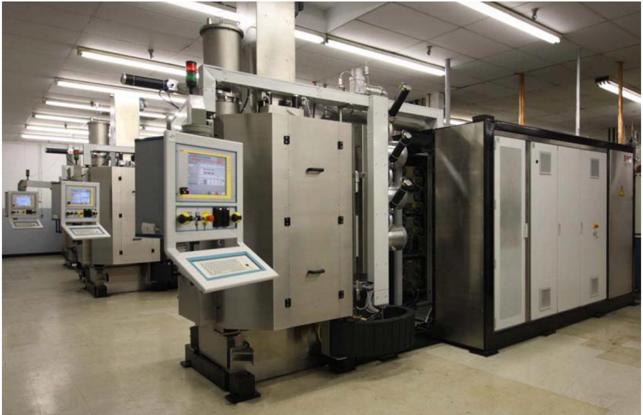
Figure 1—Me-DLC and C-DLC coating chamber line at the Richter Precision Inc, East Petersburg, Pennsylvania facility.
