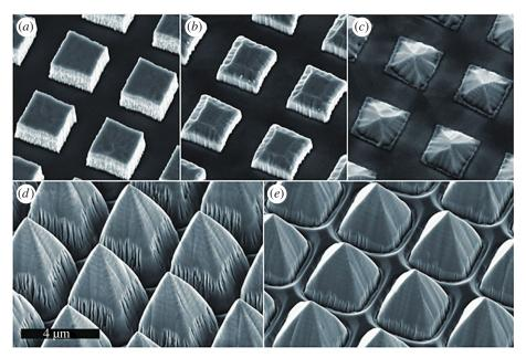
**Figure 1.** Examples of CVD diamond films patterned using dry etching methods. In (a-e), a variety of different etch processes and mask preparations have been used to define features with different sizes, shapes and sidewall slopes. Similar dry etch methods can be used to pattern diamond films into almost any desired shape, including needles, columns, pyramids, etc. Reproduced from [25] under CC-BY licence. (Online version in colour.)
