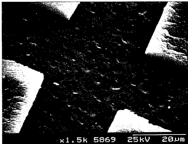
Fig. 5. SEM image showing a small portion of a patterned a-D film on Si(100) produced by PLD through a TEM mask affixed to the substrate.
