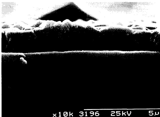
Fig. 2. Cross-section similar to that in Fig. 1, except the barrier layer here was an alloy containing 40 at.% Ge-60 at.% Si. The presence of Si has greatly improved the interface, and the diamond film is now strongly adherent.
