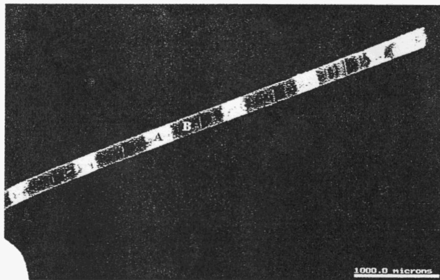
Fig. 11. Low-magnification secondary electron image of a diamond fibre showing laser irradiated area at 'B' and unirradiated area at 'A'.
