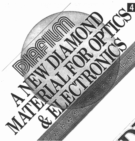
Example of a high quality 10cm diameter polycrystalline diamond ('DIAFILM') window which was grown by CVD, then removed from its substrate and all but its periphery lapped and polished to a surface roughness <5nm
