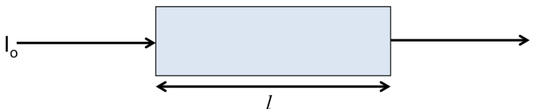
Fig. 2.8. Representation of an absorption experiment, where I_0 and I represent the intensity of the radiation entering, and leaving an absorbing material of length l .
